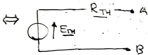
$$R_{TH} = \frac{Z_1 Z'_1}{Z_1 + Z'_1} + Z_1 = \frac{2Z_1 Z'_1 + Z_1^2}{Z_1 + Z'_1} \quad E_{TH} = V R_{TH}$$
