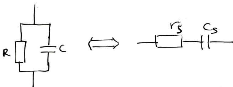
$$\underline{Z} = \frac{R}{1 + j R C \omega} = \underline{Z}' = r_s + \frac{1}{j C_s \omega} = r_s - j \frac{1}{C_s \omega}$$
