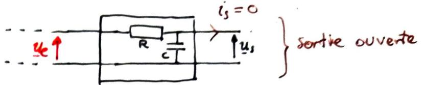
$$\begin{aligned} \underline{H} &= \frac{\underline{u}_s}{\underline{u}_e} \\ &= \frac{1}{R + \frac{1}{jC\omega}} \\ &= \frac{1}{1 + jRC\omega} \end{aligned}$$
