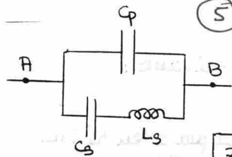
$$\frac{1}{Z} = jC_p \omega + \frac{1}{jL_s \omega + \frac{1}{jC_s \omega}} = j\omega \left[ C_p + \frac{C_s}{1 - L_s C_s \omega^2} \right]$$
