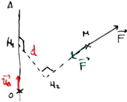
$$\begin{aligned} \mathcal{M}_\Delta(\vec{F}) &= \mathcal{M}_O(\vec{F}) \cdot \vec{u}_\Delta \\ &= \overrightarrow{OM} \wedge \vec{F} \cdot \vec{u}_\Delta \\ &= (\overrightarrow{OH_1} + \overrightarrow{H_1H_2} + \overrightarrow{H_2M}) \\ &\quad \wedge \vec{F} \cdot \vec{u}_\Delta \end{aligned}$$
