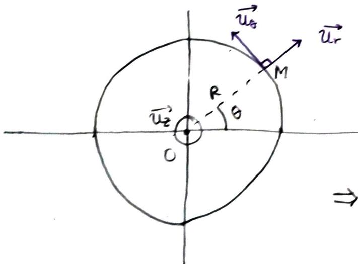
$$\begin{aligned}\begin{cases} \vec{OM} = R \vec{u}_r & R \text{ constant} \\ \vec{v} = \cancel{R \dot{\theta} \vec{u}_r} + R \dot{\theta} \vec{u}_{\theta} \end{cases} \\ \Rightarrow \vec{L}_O(M/R) = \begin{pmatrix} R \\ 0 \\ 0 \end{pmatrix} \wedge m \begin{pmatrix} 0 \\ R \dot{\theta} \\ 0 \end{pmatrix} \\ = m R^2 \dot{\theta} \vec{u}_z\end{aligned}$$
