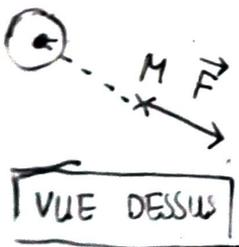
$$\begin{aligned} \mathcal{M}_\Delta(\vec{F}) &= \vec{M}_O(\vec{F}) \cdot \vec{u}_\Delta \\ &= \vec{0} \cdot \vec{u}_\Delta \\ &= 0 \end{aligned}$$
