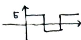
$$u_e(t) = \frac{4E}{\pi} \left( \underbrace{\sin(2\pi f_0 t)}_{\text{fondamental}} + \underbrace{\frac{\sin(2\pi 3f_0 t)}{3} + \frac{\sin(2\pi 5f_0 t)}{5} + \dots}_{\text{harmoniques}} \right)$$
