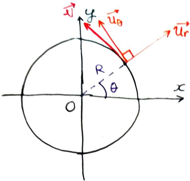
$$\begin{aligned} \vec{OM} &= R \vec{u}_r \\ \Rightarrow \vec{v} &= R \dot{\theta} \vec{u}_\theta \\ \Rightarrow \vec{a} &= -R \ddot{\theta} \vec{u}_r + R \dot{\theta} \dot{\vec{u}}_\theta \\ &= -R \omega^2 \vec{u}_r + R \dot{\omega} \vec{u}_\theta \quad \omega = \dot{\theta} \\ &= -\frac{v^2}{R} \vec{u}_r + \frac{dv}{dt} \vec{u}_\theta \quad \frac{v}{R} = \omega \end{aligned}$$
