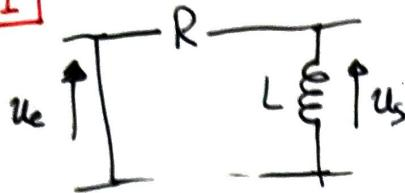
$$\underline{H} = \frac{jL\omega}{R+jL\omega} = \frac{j\frac{L}{R}\omega}{1+j\frac{L\omega}{R}} = \frac{j\frac{\omega}{\omega_0}}{1+j\frac{\omega}{\omega_0}} \quad \text{avec } \omega_0 := \frac{R}{L}$$
