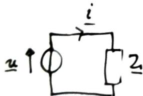
$$\begin{aligned} u &= U_m e^{j\omega t} \\ i &= I_m e^{j(\omega t + \varphi)} \end{aligned}$$
