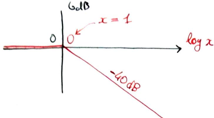
$$H = \frac{1}{1-x^2+3jx} \quad \text{de la forme} \quad \frac{1}{1-x^2+j\frac{x}{Q}} \quad \text{ici } Q = \frac{1}{3}$$
