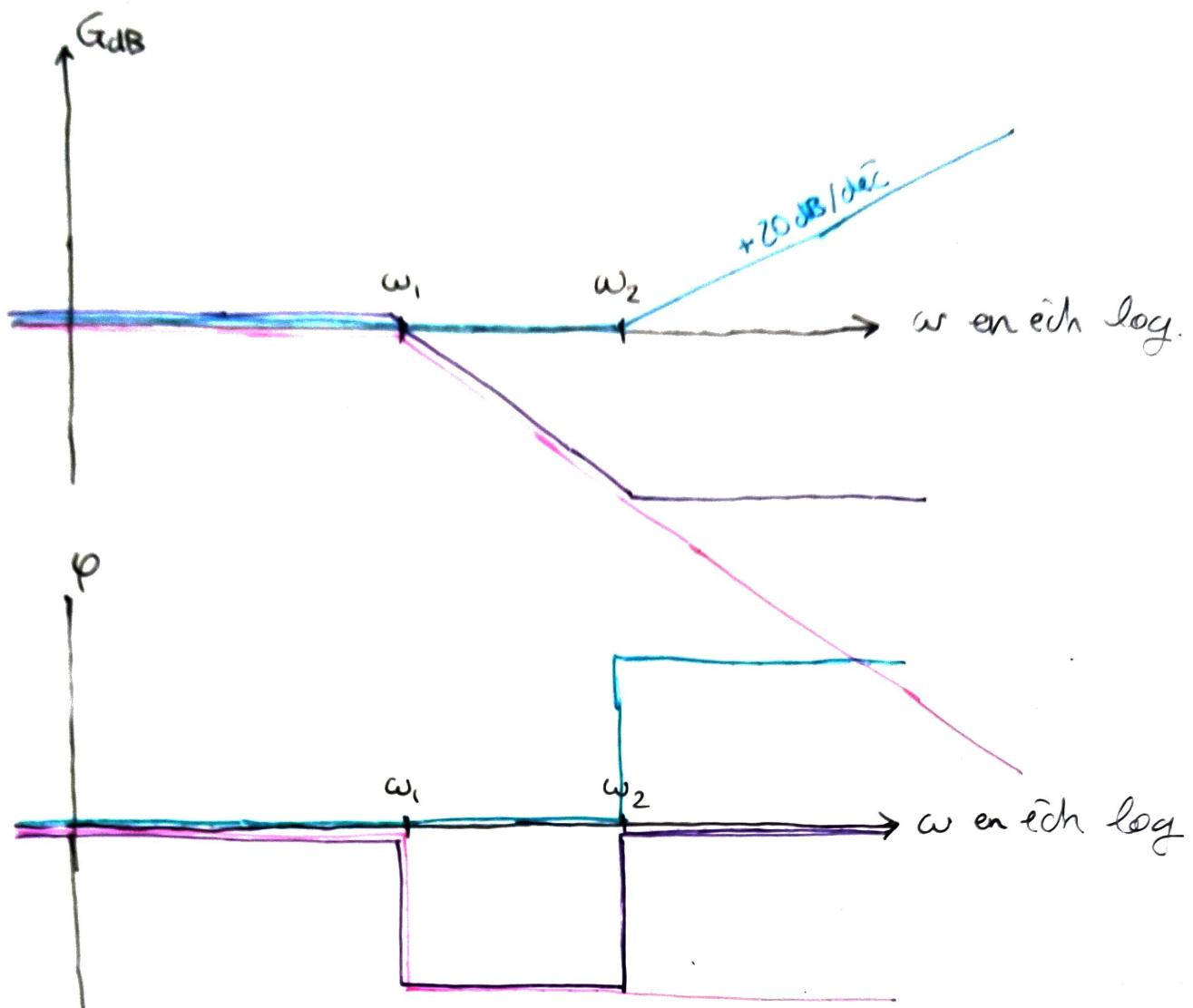
$$H = \frac{H_2}{H_1} = \frac{1 + j \frac{\omega}{\omega_1}}{1 + j \frac{\omega}{\omega_2}}$$
